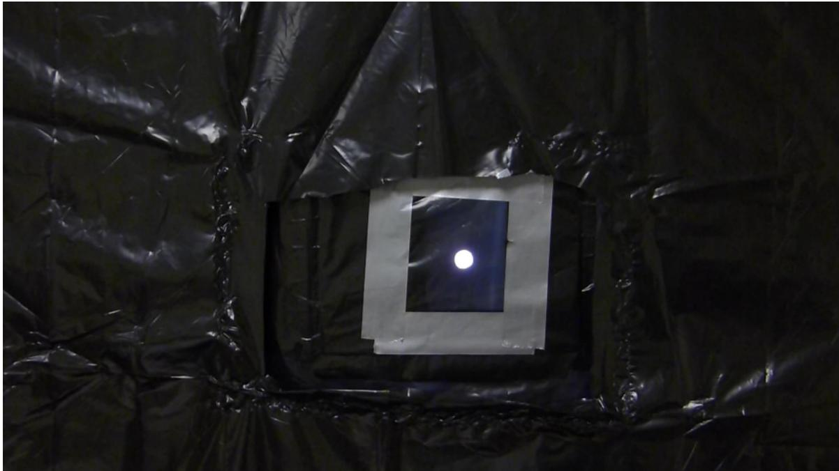
**Figure 2.** Aperture unit taped over a rectangular opening in the large black sheet to easily exchange aperture sizes.
