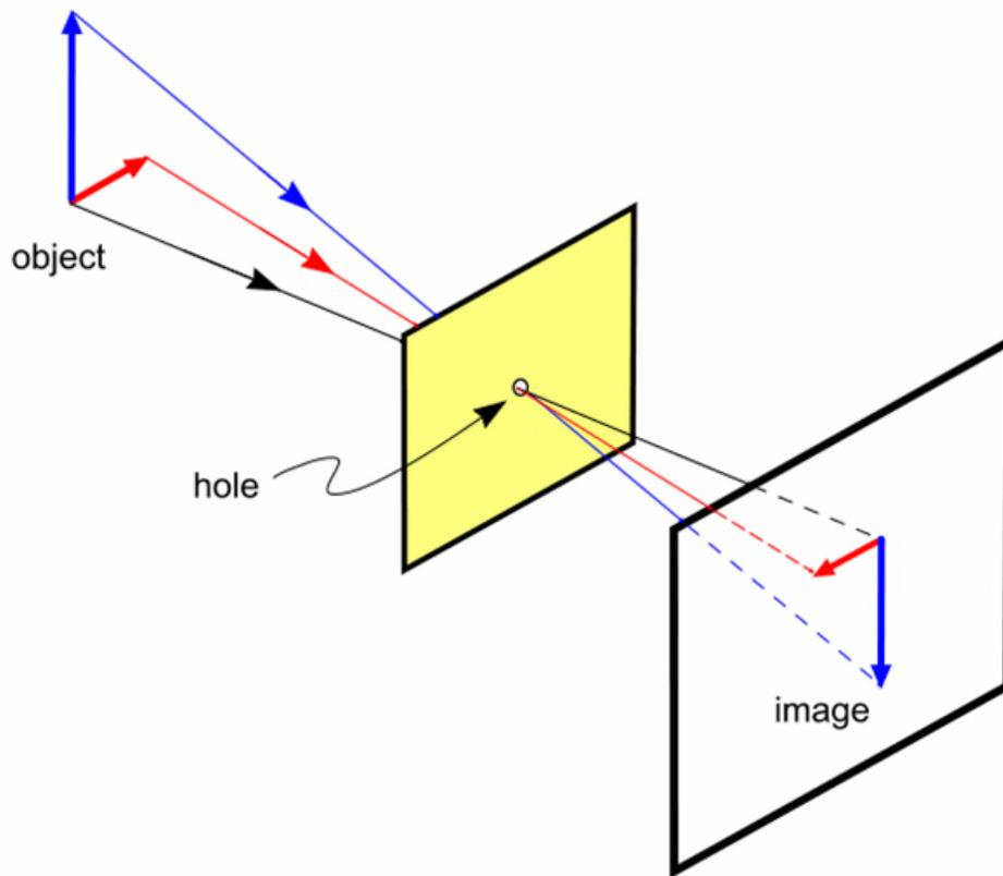
**Figure 1.** Ray diagram of a camera obscura.
