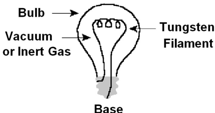
**Figure 1.** Simple sketch of incandescent light bulb.
