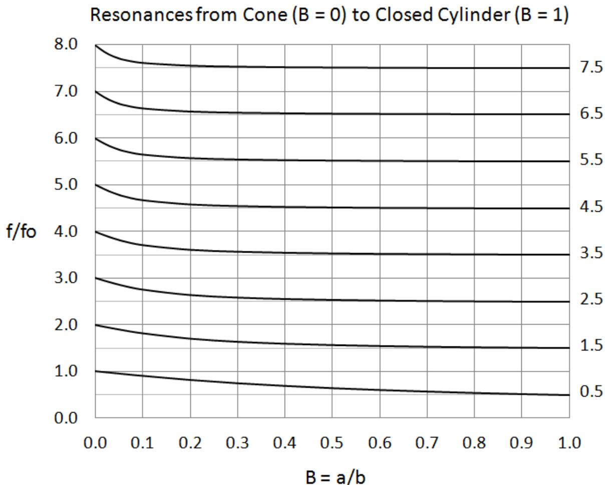
Figure 4. Plots of the first eight resonance frequencies of a conical frustum (slant length  $L$  and closed on the smaller end) relative to the fundamental frequency of an open pipe of length  $L$ . The value  $B=0$  indicates a complete cone and  $B=1$  defines a closed cylindrical pipe.
