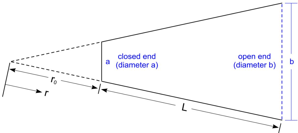
Figure 2. Conical frustum closed at the smaller left end where the pipe diameter is  $a$  and open at the larger right end where the pipe diameter is  $b$ . The slanted length of the conical pipe is  $L$ . The figure is not drawn to scale since  $b$  should be less than  $\frac{L}{5}$  as explained in the first section of this paper.
