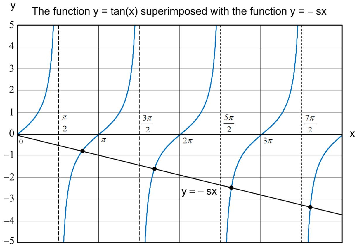
Figure 3. Solving the transcendental equation  $\tan x = -sx$  by superimposing the graphs  $y = \tan x$  and  $y = -sx$ . The intersection points are the solutions for the values of  $x$ , from which the resonance frequencies are found:  $f = \frac{x}{\pi} f_o$ .
