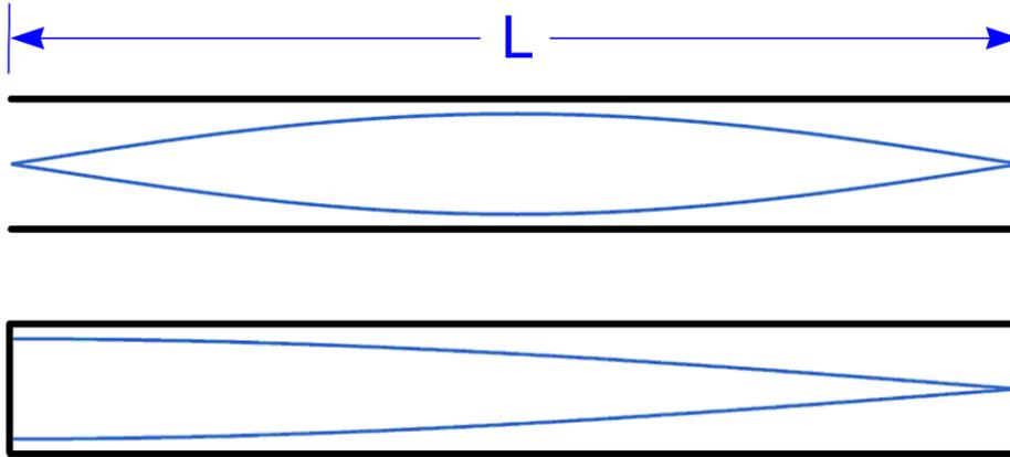
Figure 1. First longitudinal standing waves for an open pipe and a closed pipe. The curves indicate the pressure changes relative to equilibrium pressure for the longitudinal waves.
