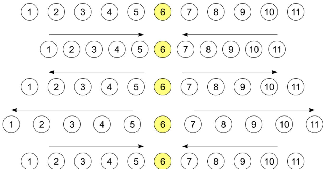
Figure 3a. The choreography for dancing the fundamental in an open pipe. Students at each end first move inward to squeeze student 6 at the center and then move outward to stretch student 6.
