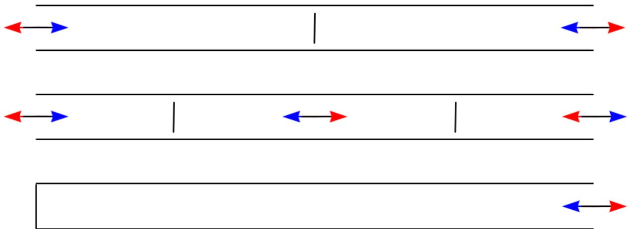
Figure 2. Schematic for the fundamental mode of an open pipe (top), the second harmonic mode of vibration for an open pipe (middle), and the fundamental mode for a closed pipe (bottom).
