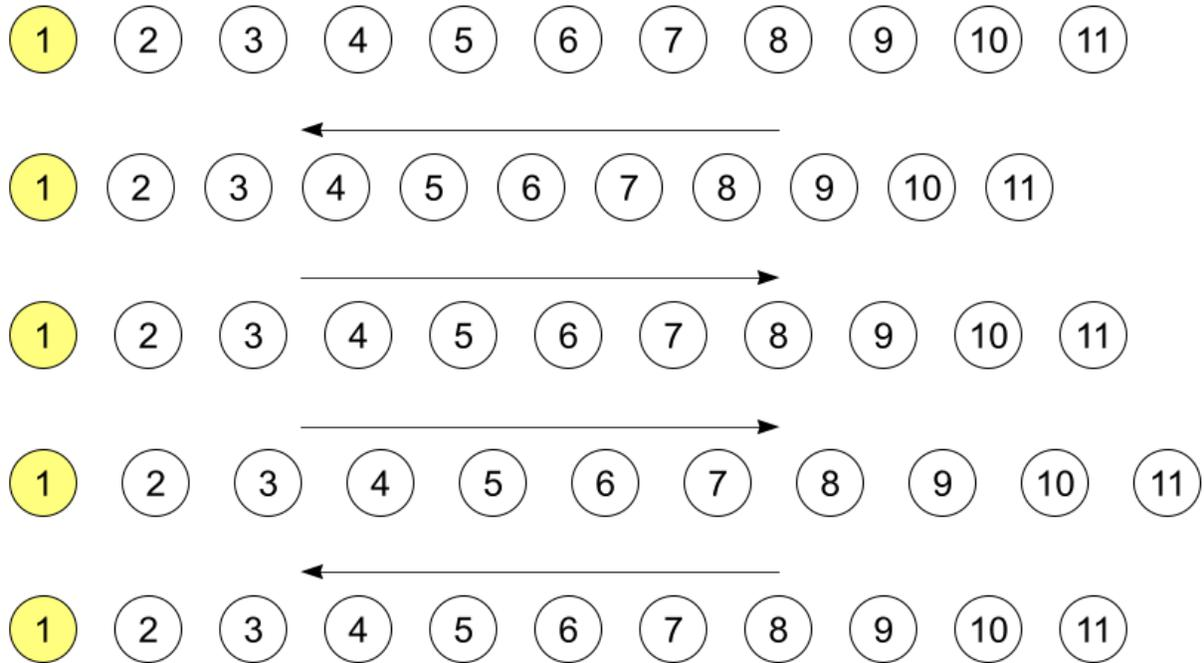
Figure 3c. The choreography for dancing the fundamental of a closed pipe. Student 1 is a displacement node at a wall in the classroom. The other students first move in to squeeze student 1 and then move out to stretch student 1.
