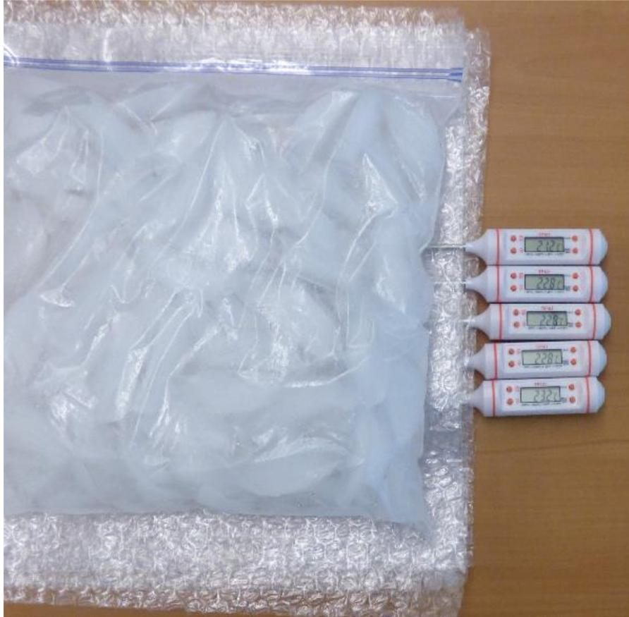
**Figure 1.** Experiment for taking temperature readings under 1, 2, 3, 4, and 5 layers of bubble wrap when ice is placed on top.
