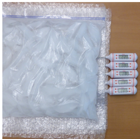
Figure 1. Experiment for taking temperature readings under 1–5 layers of bubble wrap when ice is placed on top.
