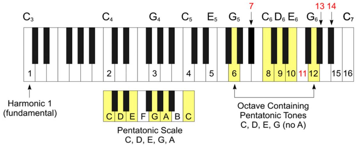
**Figure 2.** First sixteen harmonics and their best matching positions on the keyboard. The pitches of harmonics 7, 11, 13, and 14 are not very close to their respective keyboard notes. Key C<sub>3</sub> is 130.8 Hz.
