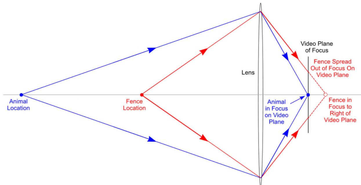
**Figure 4.** A point from the animal subject is focused as a point in the video plane of focus since the videographer has zoomed in on the animal. A point from the fence is spread out on the video plane as its point of focus lies beyond and to the right of the video plane of focus.
