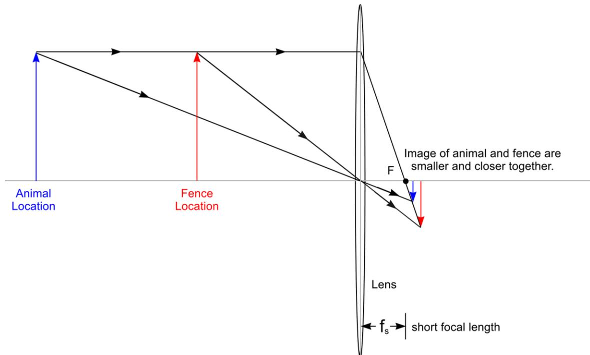
**Figure 3.** (a) Animal and fence subjects and their corresponding real images for a long focal-length lens. (b) The same subjects with their real images formed by a short focal-length lens. The images for the short focal length (figure b) are smaller and closer to each other.
