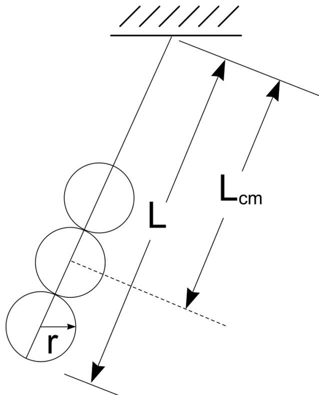
Figure 2. Model for beads forming a physical pendulum where beads are in the lower section of the pendulum and no beads are in the upper section.
