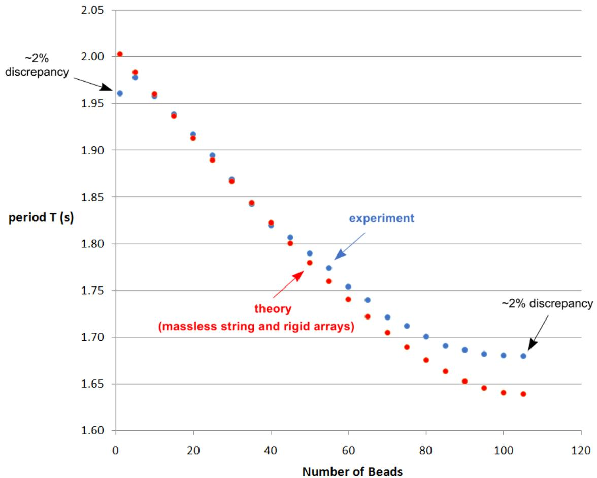
Figure 4. The experimental data compared to theory based on a massless string and rigid bead arrays. The 2% discrepancy for the simple pendulum arises since the string mass is not negligible for one bead. The 2% deviation for 105 beads is due to the flexibility of the beam.
