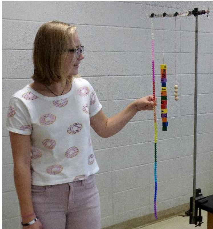
Figure 1. Coauthor Chloe Hawes with three types of beads. For each case, the experiment started with beads stacked from the bottom up to the pivot point with a very small space near the pivot to allow for free swinging. Beads were gradually removed from the top, keeping the total length of the pendulum constant for each series of experiments.
