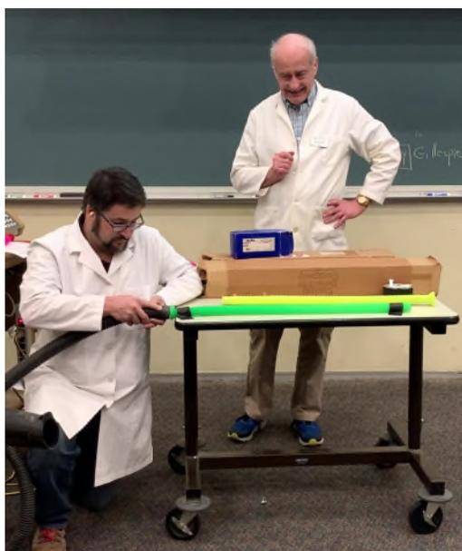
**Figure 1.** (a) Corrugated tube placed over vacuum cleaner hose. (b) Vacuum cleaner hose isolating higher harmonics as it is brought closer to the tube. Photos Courtesy Noah Michael
