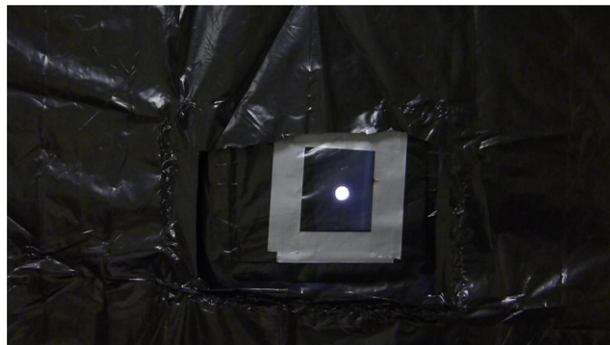
Figure 2. Aperture unit taped over a rectangular opening in the large black sheet to easily exchange aperture sizes.
