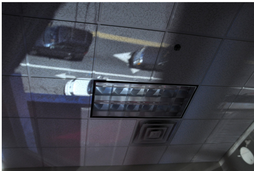
Figure 4. Photograph of camera obscura ceiling image by Halima Flynt. Digital camera info: exposure time 30 s, f -number f/7.1 , sensitivity ISO 800, wide-angle f = 27 mm (35 mm film equivalent).
