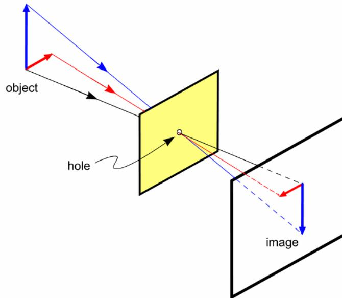
**Figure 1.** Formation of image on a screen as light passes through a small hole. If the hole is too small, diffraction will cause the image to blur. If the hole is too big, light from a single point on the object reaches many points on the image screen, causing blur.
